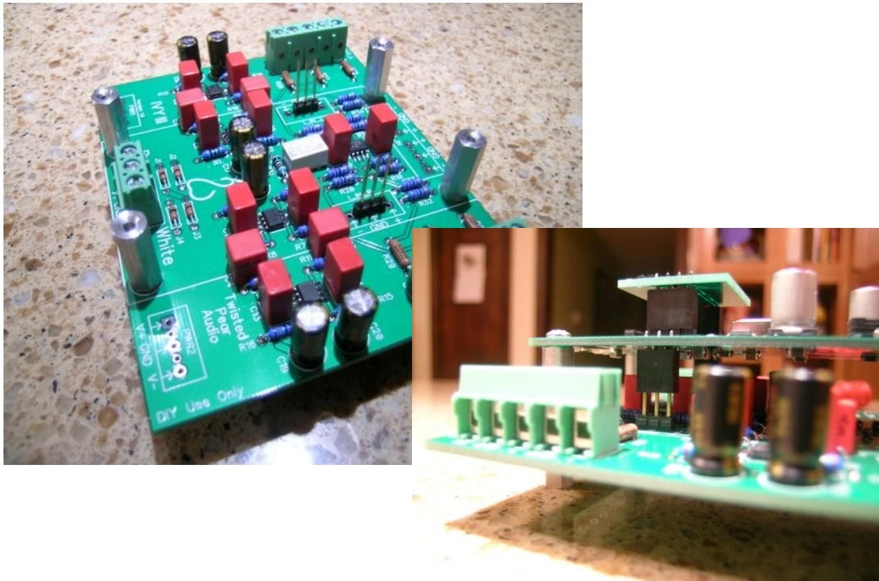
Notice that one set of current input headers physically lines up with the Buffalo-II current output headers when the Buffalo-II is placed over the IVY-III. Stacking with the Buffalo II using male and female .1" (2.54mm) pin-headers will give you the shortest possible signal path from the DAC yielding the best results (included in the complete kit).
