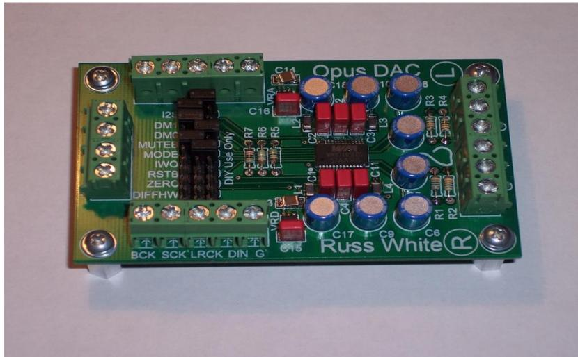
Figure 1, A populated DAC PCB setup for 24 bit I2S input and stereo output with no deemphasis. Notice just the first 6 jumpers are used.
