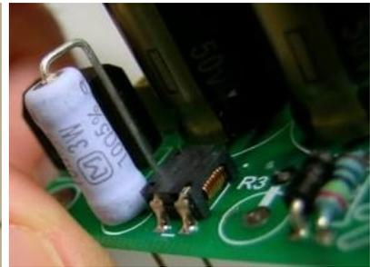
Resistors are normally marked with a rectangle on the PCB, and often designated with an R... number. See R1 to R8 on the lay-out of the Placid.
