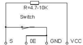
By closing the switch, S is connected to ground. Connector A will be switched to B1. When the switch is open A will be switched to B2.
