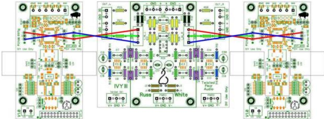
Bridging the outputs increases the signal that goes into the I/V stage. Depending on the I/V stage it may be required to correct the gain of the I/V stage, as described in the next section.
